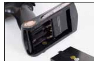
Remove the battery cover and put in 4 AA size batteries.
