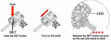
**Note2:** If you don't release the 'SET' key as soon as the red LED begins to flash, the ESC will enter the program mode, in such a case, please switch off the ESC and re-calibrate the throttle range again from step **A** to step **D**.
