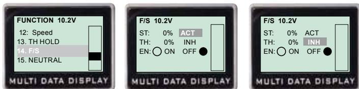
This function does not work in PPM mode. If the RF signal loss, it should occur the receiver adjust the Steering or Throttle or both to a preset value.
