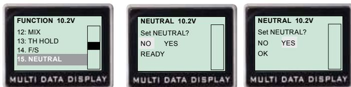
This function can calibrate the neutral of the STEERING wheel or THROTTLE trigger.
