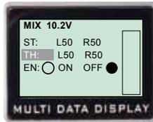
This function allows customer to apply mixing between the steering, throttle, and channel 3 channels. There are main channel and sub-channel in the MIX selection. The servo travel value of the sub channel is changed along with the change of the main channel according to the setting rate.
