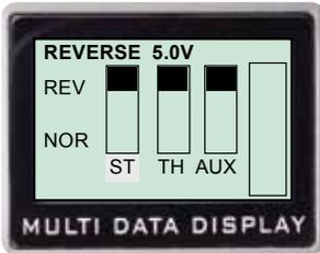
This function reverses the direction of operation of the servos related to transmitter steering, throttle, and channel 3 operation.
