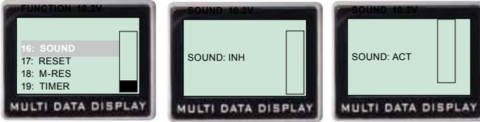
This function can open or close the buzzer sounding.
