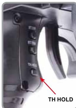
the engine. It can be performed for accident braking. When pressing the switch, throttle trigger doesn't work until the switch is pressed again.
