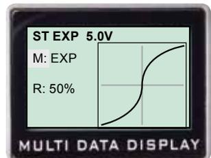
This function is used to change the sensitivity of the steering servo around the neutral position. It has no effect on the maximum servo travel.
